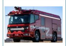
A range extended electric fire appliance produced by Rosenbauer has been in operation in Los Angeles since May 2022.
